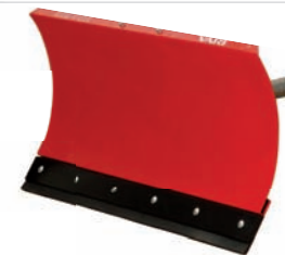
ASR-1000 dozer blade + adjustable holder and lifting lever working width: 100 cm spring suspension, rubber edge product No. 4328
