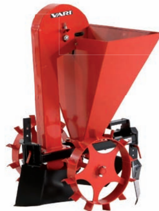
SB-40 potato planter automatic single-row cup type potato planter mounted to the front holder with bin holding up to 20 kg wheel gauge 61 cm product No. 4363
