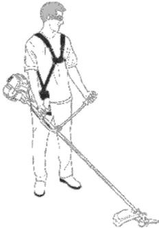
After the brush cutter/trimmer is started, hang it on the harness and grasp the handlebars properly.
