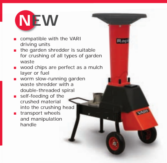
RAPIDO wood chipper Recommended engine power: 3,5 – 6,5 HP Clutch diameter: 80 mm Maximal diameter of crushed material: up to 55 mm Approximate size of wood chips: 20 mm Article no.: 4449
