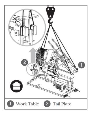
The processor can be lifted with ropes suitable to support its weight. When lifting the machine, firmly tie up the ropes at work table (1) and tail plate (2).
