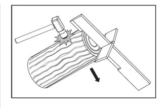
Open the main steel mesh, dismantle the protecting wire net and take out the jammed log and cross wedge.
