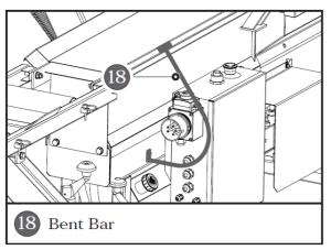
Fix the bent bar (18) to machine case and machine body with three pieces of M16x10 screws as shown.
