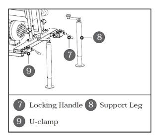
Loosen the locking handles (7) in the anticlockwise direction. Install the support legs (8) to U-clamps (9). Fasten the locking handles in the clockwise direction. Lower the machine on the ground and release the ropes. Loosen the locking handles in the anti-clockwise direction to adjust the support legs on the same level of the transport wheels until processor is level. Fasten the lockina handles the clockwise in direction.
