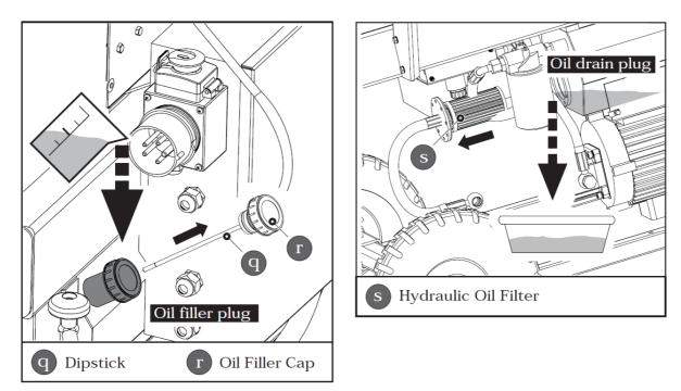
Use a drain pan to aid in the removal of all used oil and particles.
