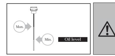
Read dipstick to determine the maximum and minimum of the oil level. Low oil can damage the oil pump. Overfilling can result in excessive temperature in the hydraulic transmission system.
