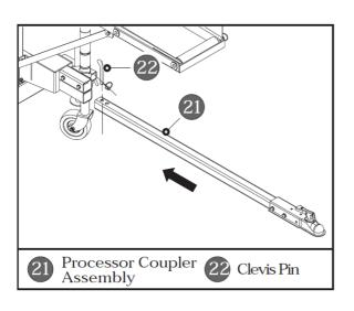
Install the processor coupler assembly (21) into the connecting piece. Line up the holes in the processor coupler assembly and the connecting piece. Insert the clevis pin (22) through the holes in the processor coupler assembly and the connecting piece. Insert lock pin through the hole in the clevis pin to secure it.
