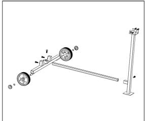
4) Put both stand legs on the log splitter shanks (position 1), then seat the log splitter on the stand frame.
