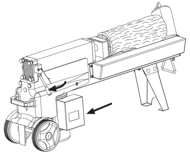
This log splitter is equipped with %ZHB+control system that requires to be operated by both hands of the user . left hand controls the hydraulic control lever while right hand controls the pushbutton switch. The log splitter will freeze upon absence of either hand. Only after both hands release the controls, the log pusher starts to return backward to the starting position.
