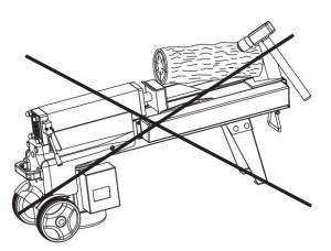
Do not try to knock the jammed log off. Knocking about will damage the machine or may launch the log and cause accident.
