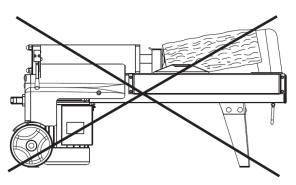
Break log in the direction of its growing grain. Do not place log across the log splitter for splitting. It may be dangerous and may seriously damage the machine. Do not attempt to split 2 pieces of logs at the same time. One of them may fly up and hit you.
