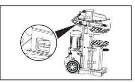
5. Bolt the control lever and guard assy in position with bolts, washers and nuts.
