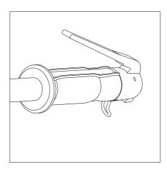
**Position 3** – is used to switch off the engine in critical situations or after the end of work. The engine will be switched off at all times after the safety ignition switch lever on the left grip of handlebars has been released; taking off hand from the handrail will do. Wire latch must be at all times released – see Warning in the description of Position 2.
