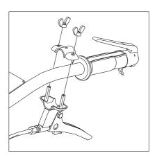
After the driving unit is installed, mount the wheel drive clutch lever on the left side of the handlebars (in front of the safety switch). Unscrew the butterfly nuts, take the lever holder off, place the lever in front of the left rubber handle, put on the lever holder and screw the butterfly nuts.
