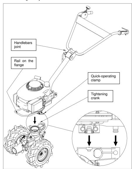
Release the tightening crank which retains the guiding handles swivel holder pivot on the gearbox.
