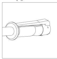
**Position 1** – is used in starting the engine, in adjusting engine speed or in a short-time machine standstill at which the engine is still running. In this position, wire latch in the lower part of the safety switch arrests the lever in pressed position.
