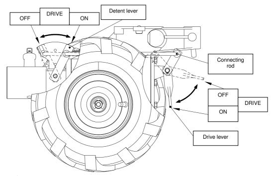
*Drive switching* – drive lever on the gearbox cover
