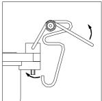
Unlock the quick-operating clamps by pushing the clamp spring loops down. Pull the clamp hooks from behind the pins and turn them aside, so that they are not in the way when taking the DU off.
