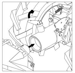
Move the lever (operating the detent pin) on the gearbox flange up – the detent pin slides into the boss in the collar. Slide the accessories drive into the gearbox flange, all the way to the drive step.
